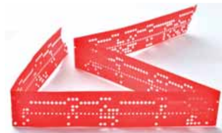
Perforated tape used in the 1970s -1980s
