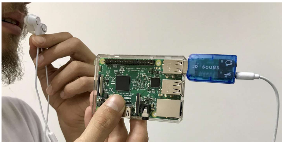
Fig. 2: Alternative use of earphones as audio input device on Raspberry Pi.
